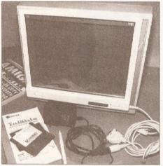
TouchWindow is attached to your monitor simply by using self-adhesive velcro tape
